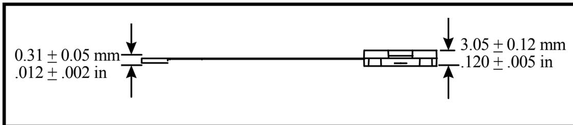
Figure 4-3. CyberDisplay™ 320 Display Dimensions Viewing Area
