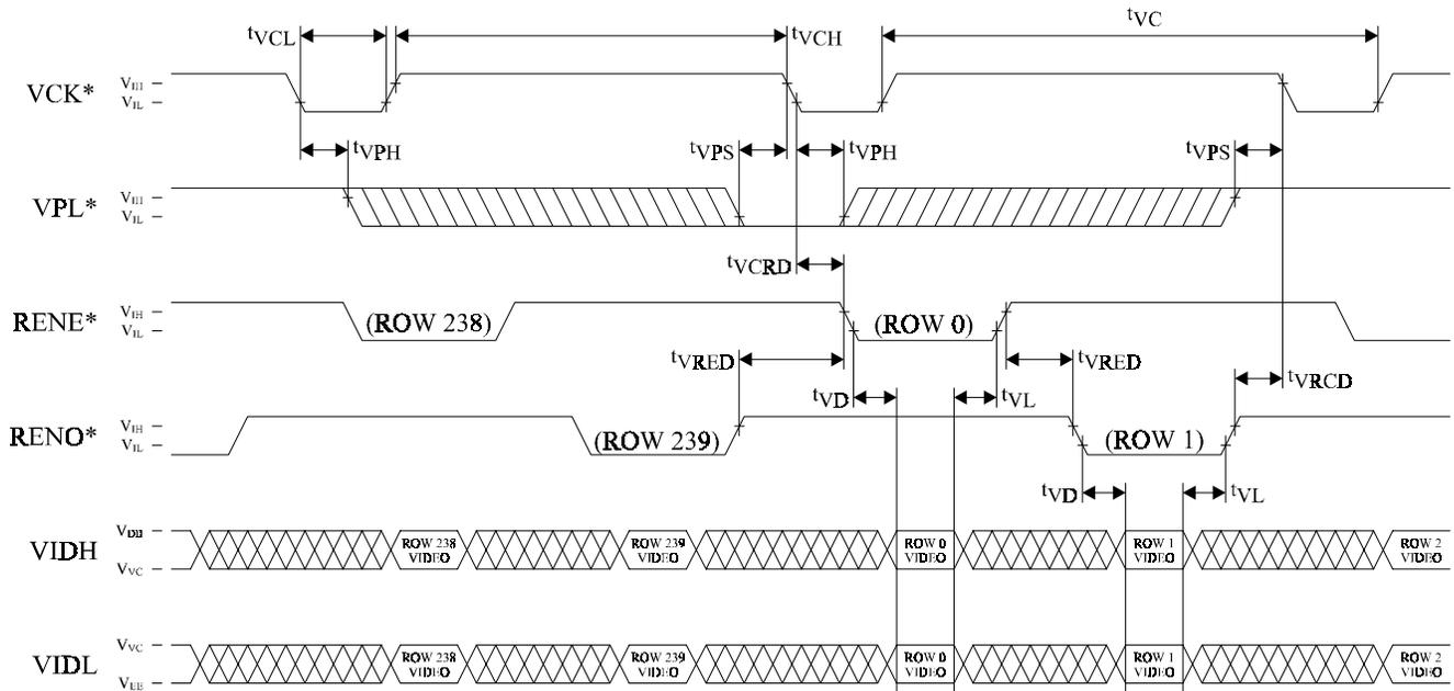
**Figure 3-3: Column Inversion Timing**
