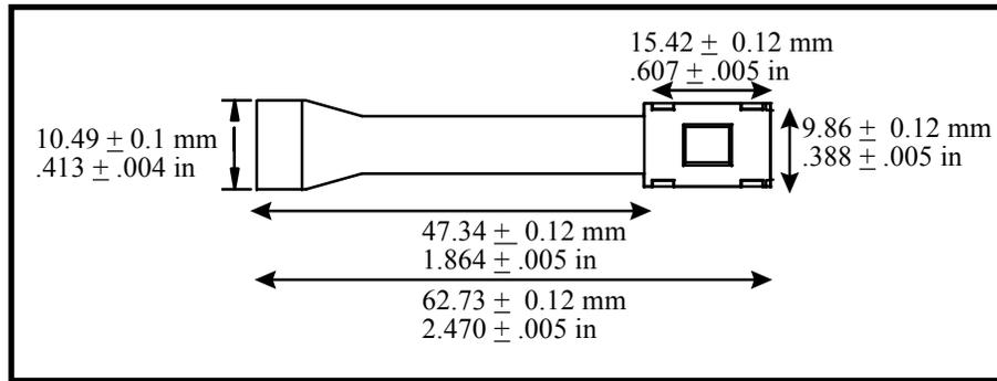
Figure 4-2. CyberDisplay™ 320 Display Dimensions Side View
